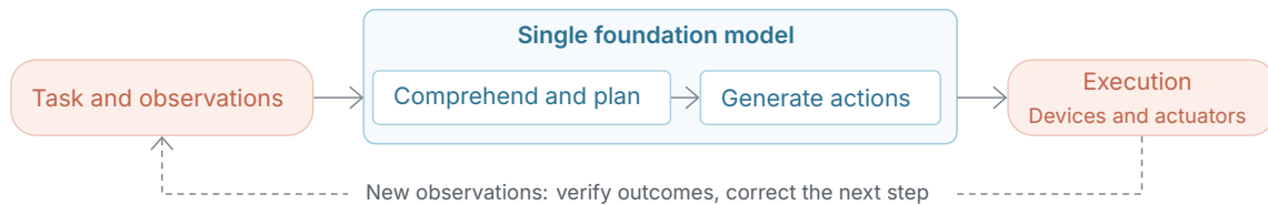
Figure 15. Brain and cerebellum become one: a single foundation model comprehends the task, generates actions, and continuously corrects course from execution feedback.
